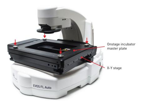
Assemble the Stagetop Environmental Chamber 1. Place the incubator chamber on the onstage incubator master plate and secure it in place using the four 2.0-mm hex screws (indicated by red arrows).
