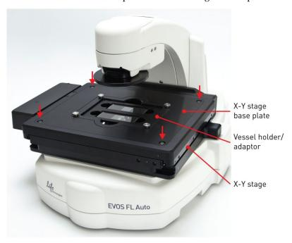
2. Secure the onstage incubator master plate to the X-Y stage using the four thumb screws (indicated by red arrows).
